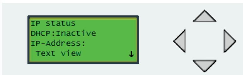
DHCP (Dynamic Host Configuration Protocol), The Dynamic Host Configuration Protocol is a standardized networking protocol used on Internet Protocol networks for dynamically distributing network configuration parameters, such as IP addresses for interfaces and services.
