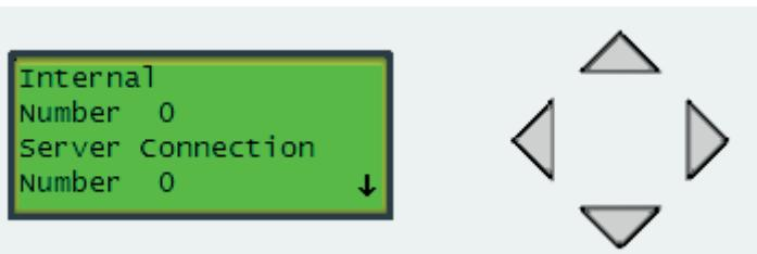
Shows number of internal and server connection errors (se 4.1.1.1), not manoeuvrable.
