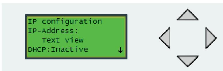
IP-address: Current IP-address, not manoeuvrable
